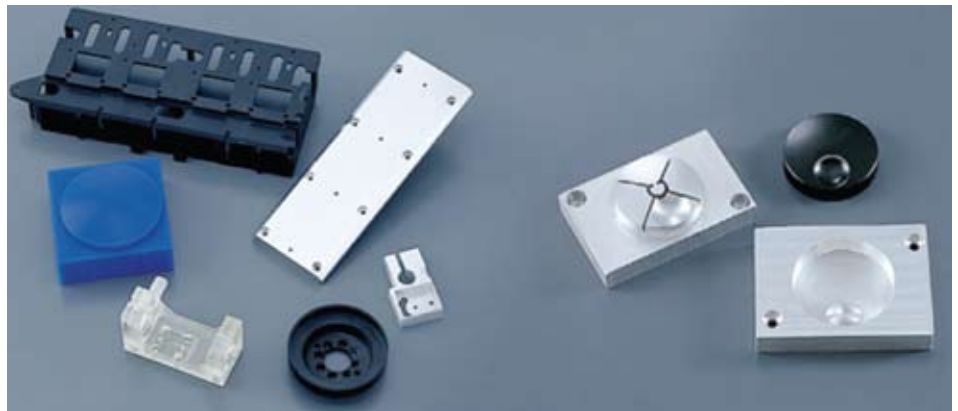
Short-run industrial parts, prototypes and molds milled with SRP on wax, aluminum, ABS, Acetal and acrylic.
