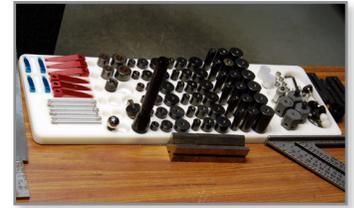
Modular clamps were used in the past to hold first articles during inspection.
