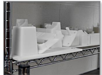
Oreck has built many FDM fixtures for CMM inspection.
