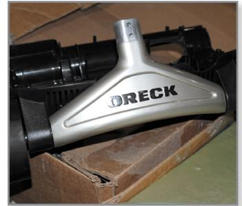
Assembly line-yoke installed on vacuum cleaner base.
